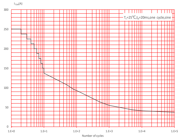
FIG.5: Non-repetitive surge peak on-state current for a sinusoidal pulse with width t_p < 20ms , and corresponding value of I^2t ( di/dt < 100A/\mu s )
